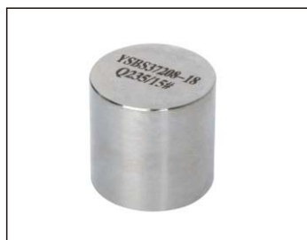
15# carbon steel control sample( optional )
